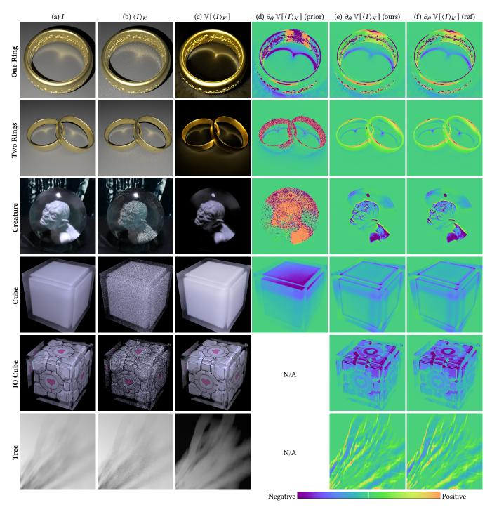
Fig. 3. **Validation**: We compare derivative estimates of rendering variances. (a) Converged path-tracing results. (b) Path-tracing results using K = 64 samples per pixel. (c) Variance of the estimator used in (b). For better visualization, we apply a sigmoid remapping to all pixel values. (d, e) Variance derivatives estimated (in equal sample and time) using the baseline [Weier et al. 2021] and our methods, respectively. (f) finite-difference references (computed in significantly more time).
