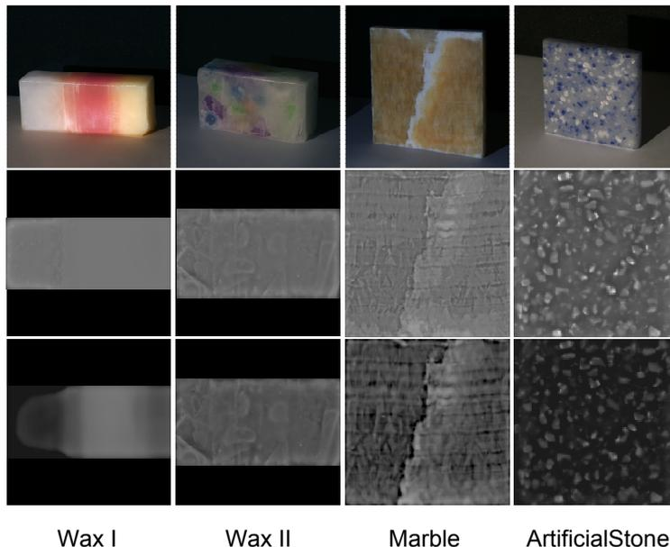
Fig. 10. Acquired material samples. Top row: real image of sample. Middle row: reconstructed  $\kappa$  along the surface. Bottom row: reconstructed  $\mu$  along the surface. The values of  $\kappa$  and  $\mu$  are scaled for better viewing.
