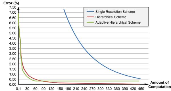
Fig. 15. Convergence speed of the three schemes. The X axis represents convergence speed in terms of 100K's of nodes that are processed.
