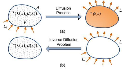
Fig. 2. Overview. (a) Rendering with forward diffusion, from the volumetric material properties ( $\kappa(x)$  and  $\mu(x)$ ) and illumination setting ( $L_i$ ) to the outgoing radiance ( $L_o$ ). (b) Model acquisition with inverse diffusion, from a set of illumination conditions ( $L_i$ ) and measured outgoing radiances ( $L_o$ ) to the volumetric material properties ( $\kappa(x)$  and  $\mu(x)$ ).
