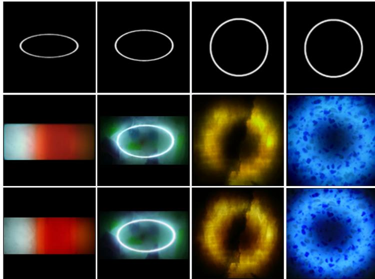
Fig. 12. Comparison of acquired models to ground truth. Top row: Illumination settings. Front lighting is applied for WaxII while back lighting is used for the other material samples. Middle row: Rendering results of volumes acquired from 16 images. Bottom row: Real images of the materials.
