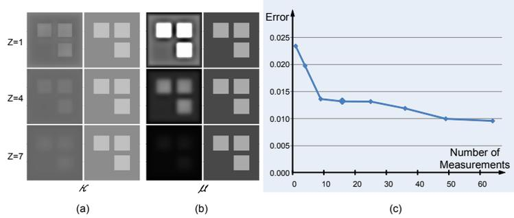
Fig. 14. Accuracy in material model acquisition. (a) Values of  $\kappa$  for the acquired material model (left) at different depth layers below the front face, and the ground truth (right). (b) Values of  $\mu$  for the acquired material model (left) at different depths, and the ground truth (right). (c) Errors of BSSRDFs computed from acquired material model using different numbers of measurements. The material model shown in (a) and (b) is acquired from 16 measurements.
