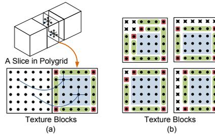
Fig. 7. Geometric primitives for nodes with different texture access patterns. (a) Three types of nodes, rendered using different geometric primitives. Each region is rendered by one primitive. (b) Geometric primitives for some texture blocks with removed nodes.
